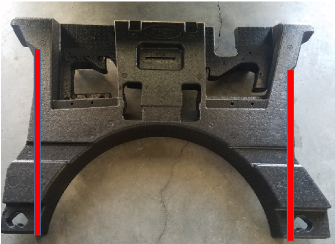
Fig.3 IMAGE SHOWING LINES WHERE TO CUT THE FOAM
