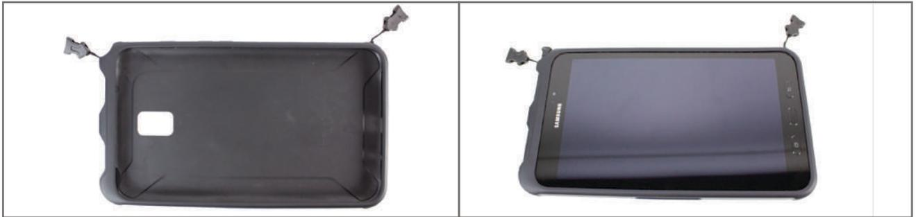
With the quick connect clips (3) installed, carefully install the Tab Active2 and stylus back into the outer case. The handle assembly (2) is now ready to be installed (see next page for Step 6).
