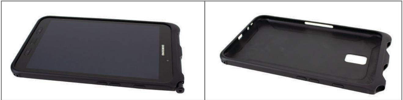
Before installation, please remove the Tab Active2 and stylus from the outer case and set them safely to the side. The mobility bundle will be installed to the outer case.
