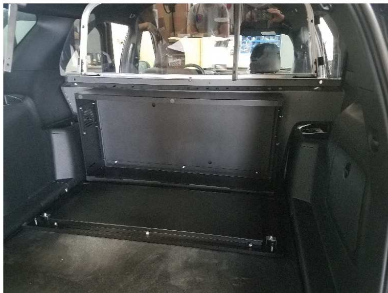
Storage box shown mounted in the back of a sport utility police vehicle with the door open to see inside.
