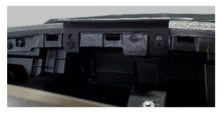
3. Attach base on to \_\_\_\_ with screws taken out in step 1. Make sure to pull base as far forward as slots allow.
