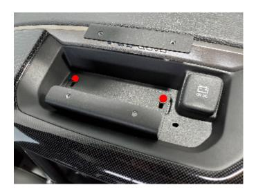
4.Loosely attach mounting bracket with (4) #10-32 hardware provided, making sure to align slots with the holes in both support and base brackets. Push plate fully towards the back and tighten all screws.
