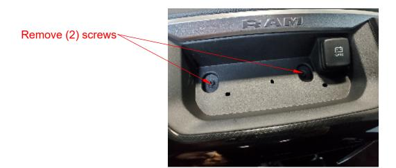
2. Remove entire front panel. Remove (2) inner most screws with a phillips head screw driver. Loosely attach support bracket with those same (2) screws. Line up front panel without fully snapping back in. Adjust support bracket to sit just on top. Fully tighten screws holding support bracket. Fully reattach front panel making sure to snap all side back in.
