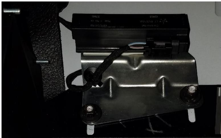
8. Front of the console is installed, align middle of the console with center stud, install the provided spacer under center leg and tighten with OEM nut (fig. 2)
