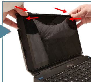
Snap Top Latch Ridge over top of Tablet.
