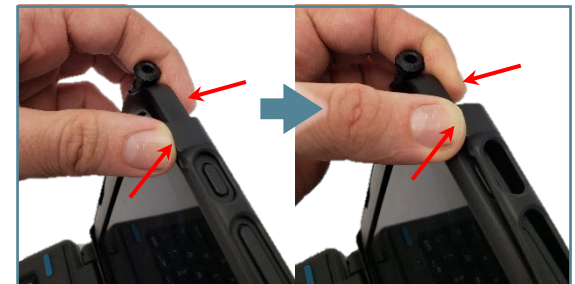
On both sides, push up on Top Latch Ridge & pull forward on back corner of Tablet.
