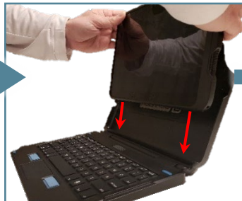
Insert Tablet into tray with Pogo Pins.
