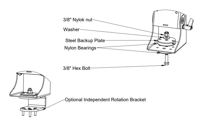
For the 7160-0220 or 7160-0928 Mongoose, use nylon bearings and steel plate as risers to clear slide
