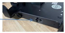
The standard mounting bracket that comes with the vehicle dock features an industry standard VESA 75mm x 75mm bolt pattern. This allows easy mounting to many pre-existing mounts as well as dedicated mounts from Gamber-Johnson. Multiple hole patterns are also present for ease of installation with various other infrastructure. Use the supplied #½-20 or #10-24 hardware for attaching it to the mount and note the orientation of the mounting plate with the large hole towards the front of the dock.
