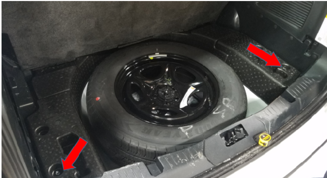
Fig.2 IMAGE FROM REAR END - 8MM BOLTS EXPOSED
