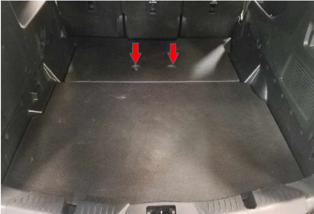
Fig.1 IMAGE FROM REAR END - TORX HEAD BOLTS
