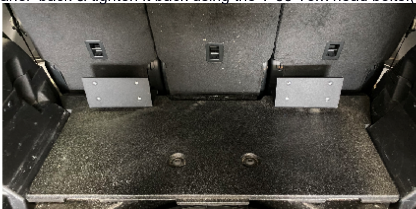
Fig.9 IMAGE FROM REAR END CARGO PANEL INSTALLED
