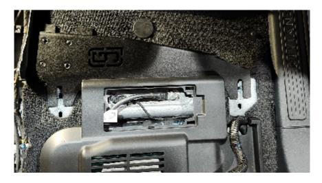
6. Re-install seat per FSM making sure vehicle base is sandwiched between seat rails and floor pan.
