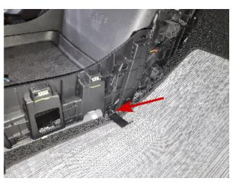
5. Set vehicle base in place, aligning slots on base with front set of seat bolt holes
