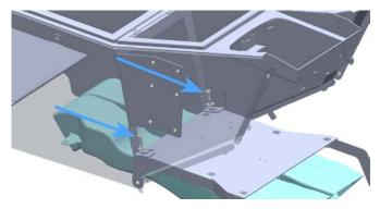
10. Route 120 volt harness and low voltage harness under console like shown
