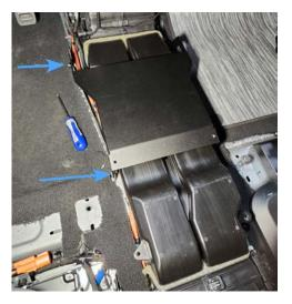
8.Carefully place the console main weldment over the electronics tray, aligning front slots with hardware installed in STEP 7. Install two OEM nuts in rear of console. **Do not fully tighten**
