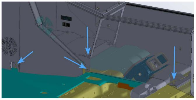
14. Install HVAC tray and fasten using provided #8 nuts and screws.
