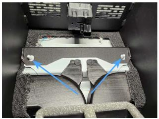
9. Fasten electronics tray to main weldment using provided 1/4-20 screws and washer. **Do not tighten**
