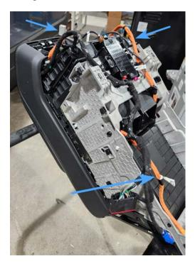
5. Remove screws holding HVAC to underside of console
