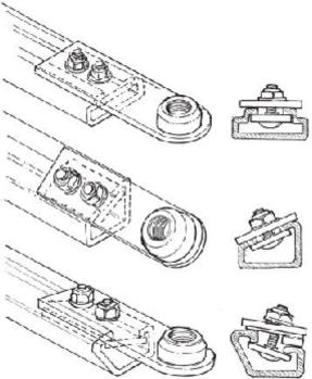
The Base Plate is placed on the top side of the chair rail and the anchor plate is placed inside. Carriage or hex head bolts are used to secure the mount.
