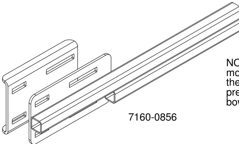
NOTE: Position the 3/8 mounting bolts as close to the pillar as possible to prevent slipping and bowing the components
