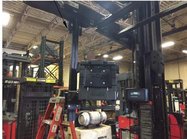
Views of pillar mount mounted on an Vertical Extension tube to position the computer equipment on the side of the fork truck
