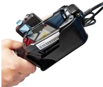
Lower the handle portion of the scanner into the dock until the spring loaded latch pops over the front surface to hold it in place.
