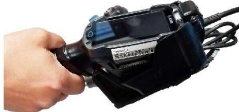
Place the top end of the scanner into the dock at approx. a 45 deg. angle
