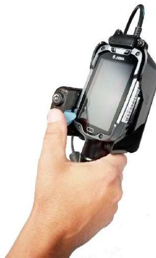
To remove the scanner, push the thumb latch to the left and pull outward on the scanner handle.
