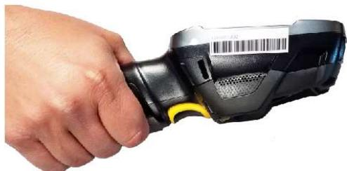
Hold the scanner as shown above with your fingers below the trigger.
