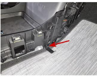
5. Set vehicle base in place, aligning slots on base with front set of seat bolt holes
