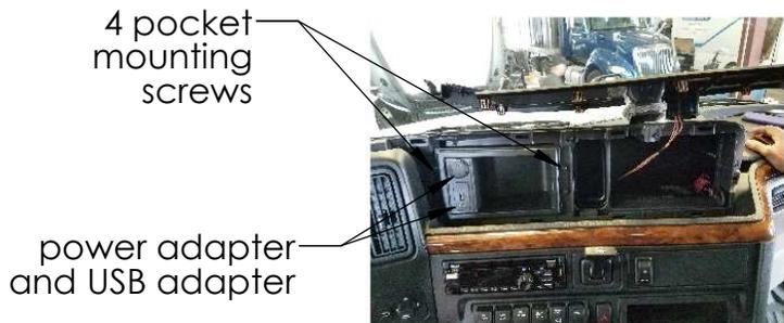
5. If the pocket has a power adapter or USB adapter, unplug the wires and remove them from the pocket. The power adapter has 2 pieces, depress the tabs inside the power adapter to separate the interior metal plug from the plastic trim ring cover.
