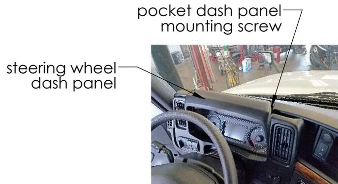
2. Remove the pocket dash panel mounting screw.
