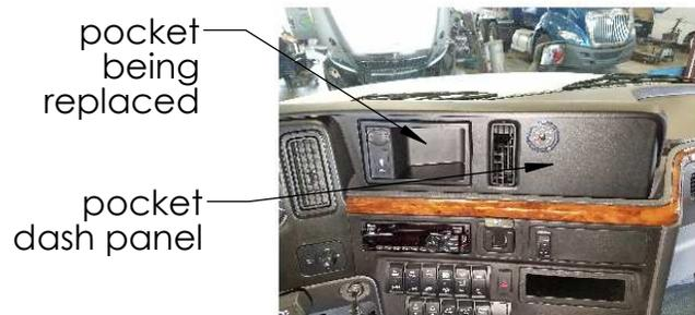
4. Remove the 4 pocket mounting screws that hold the pocket in place.
