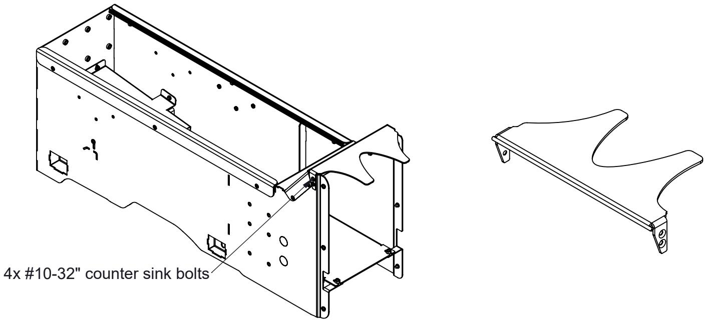
8. The driver and passenger side wings can now be installed (Items 4 and 5)
