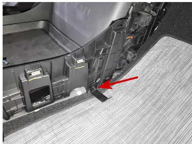
5. Set vehicle base in place, aligning slots on base with front set of seat bolt holes
