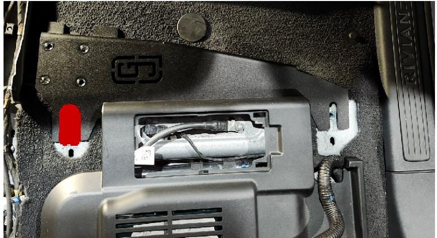
6. Re-install seat per FSM making sure vehicle base is sandwiched between seat rails and floor pan.
