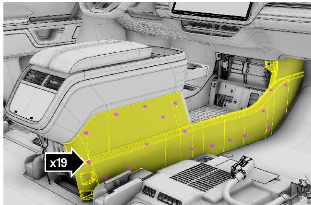
4.2 Using OEM fastener, install support bracket at indicated location. Replace trim panel
