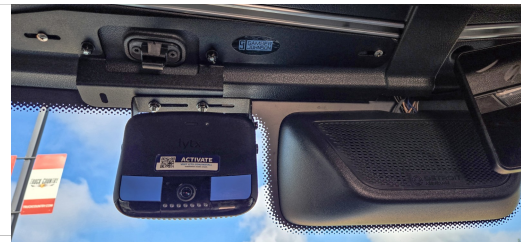
headliner mount with Lytx camera attached
