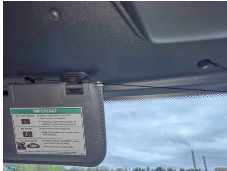
headliner mount with Samsara camera attached
