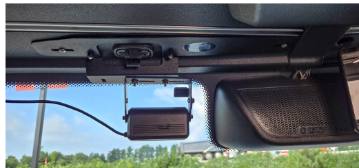
headliner mount with Samsara camera attached
