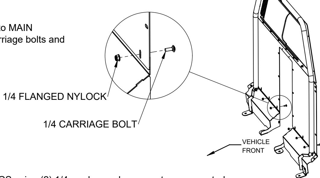
9. Install LOWER WINGS using (2) 1/4 washer and acorn nut on upper studs and (1) 1/4 washer and 1/4-20 x .5" button head screw on lower slotted hole
