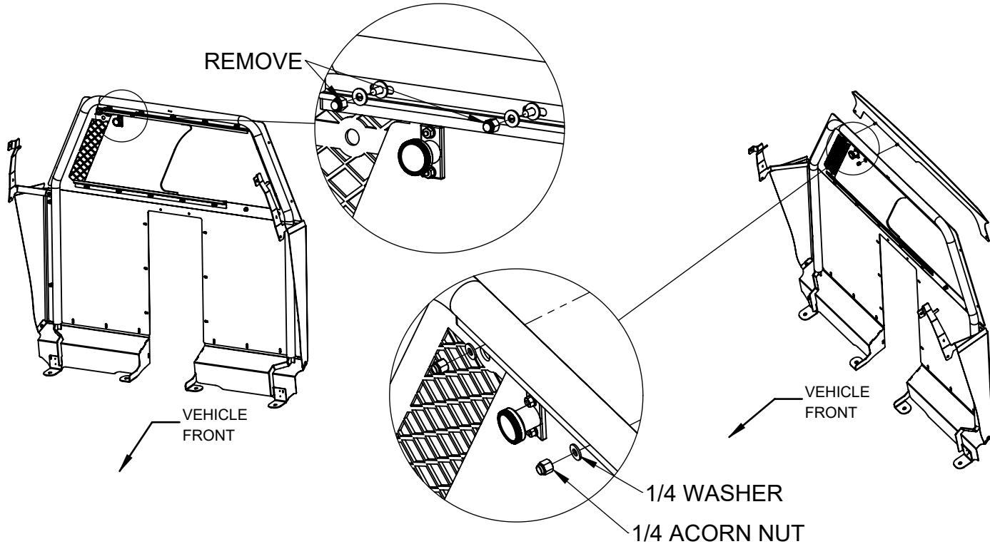
11. Install POLY WINGS using 1/4-20 x .875" button head screw, nylon washer, flat washer, and acorn nut
