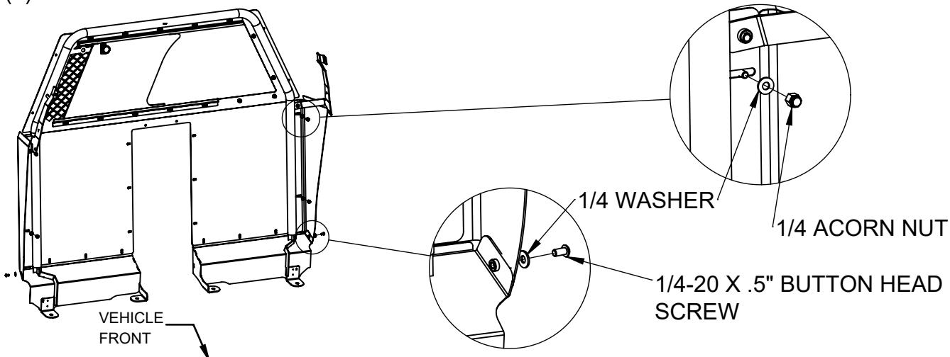
10. Remove the (2) 1/4 hardware from upper passenger side of main weldment window. Reusing (1) 1/4 wahser and acorn nut per stud, install TOP CENTER FILLER
