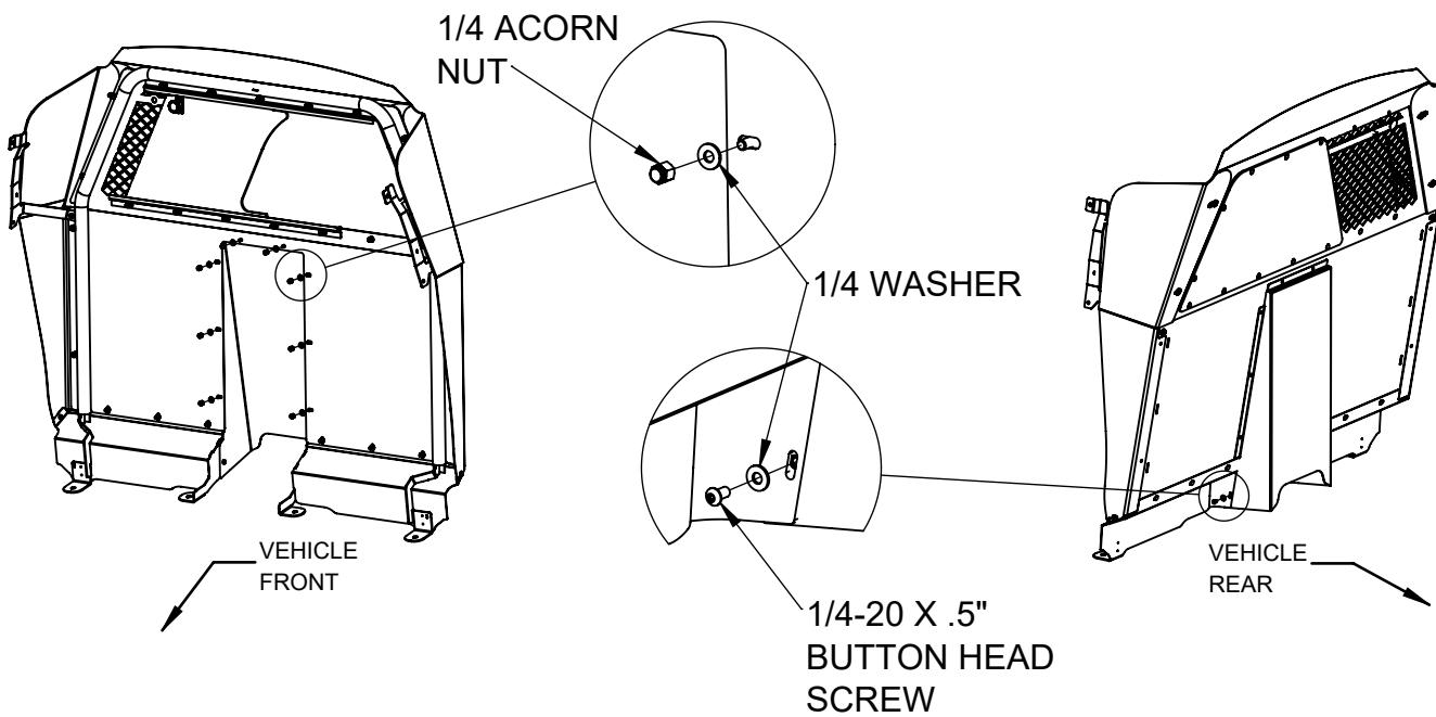
13. All fasteners can now be fully tightened. Ensure front driver and passenger seat bolts are tightened to factory specification.
