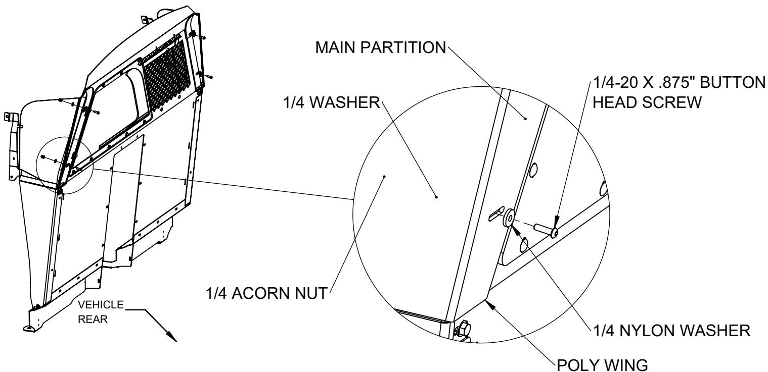
12. Install BOTTOM CENTER FILLER aligning studs it's studs with the cooresponding holes in the MAIN PARTITION. Fasten using (8) 1/4 washerS and acorn nutS on upper studs and (2) 1/4 washer and 1/4-20 x .5" button head screw on lower slotted hole
