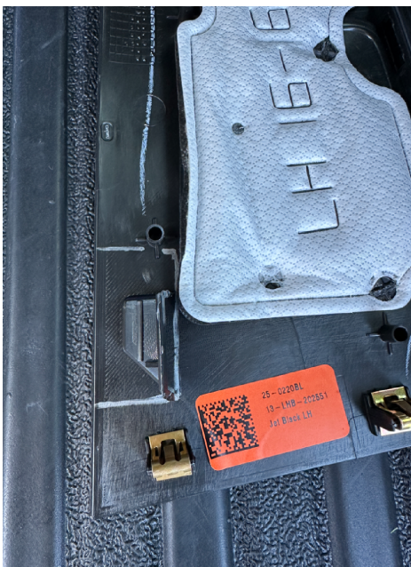
Driver side OEM trim to cut
