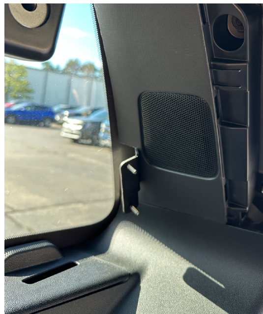
Passenger side bracket installed
