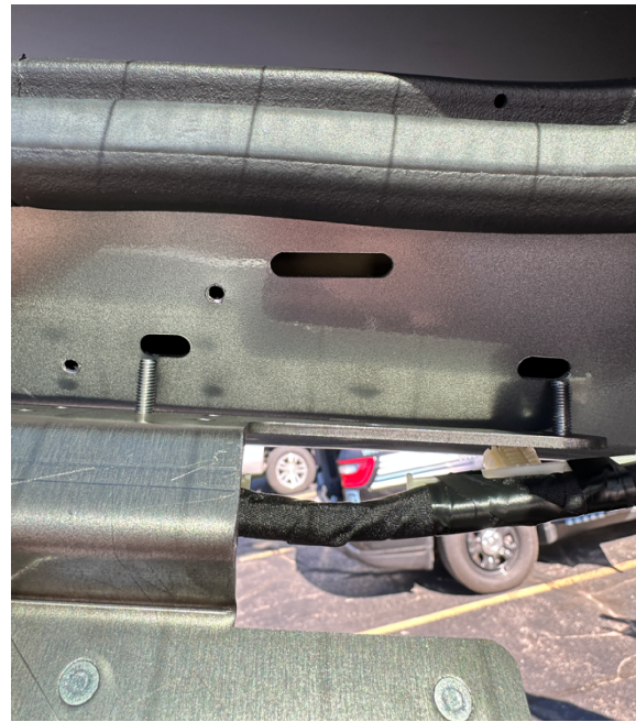
Driver side bracket being installed into slots
