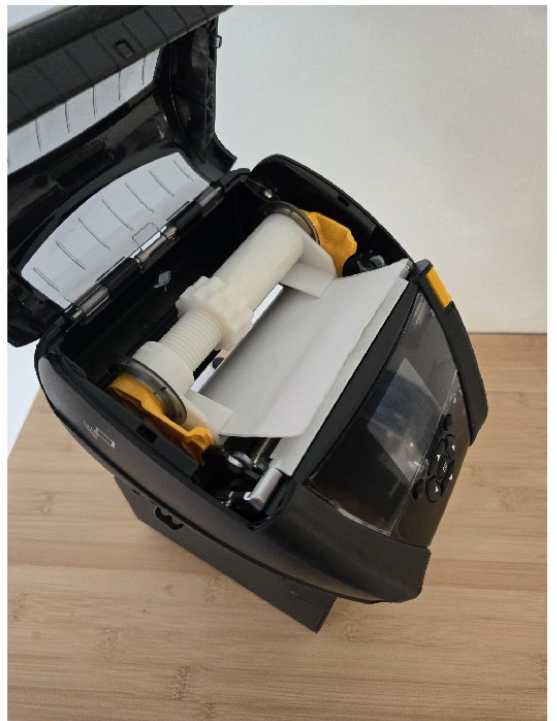
internal view of 4" wide fanfold labels being fed through the spacer kit
